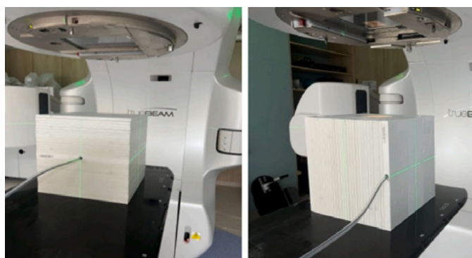
Figure 1. Slab phantom setup for CBCT dosimetry measurements using a Farmer-type ionisation chamber. Left: central position; right: peripheral position.
