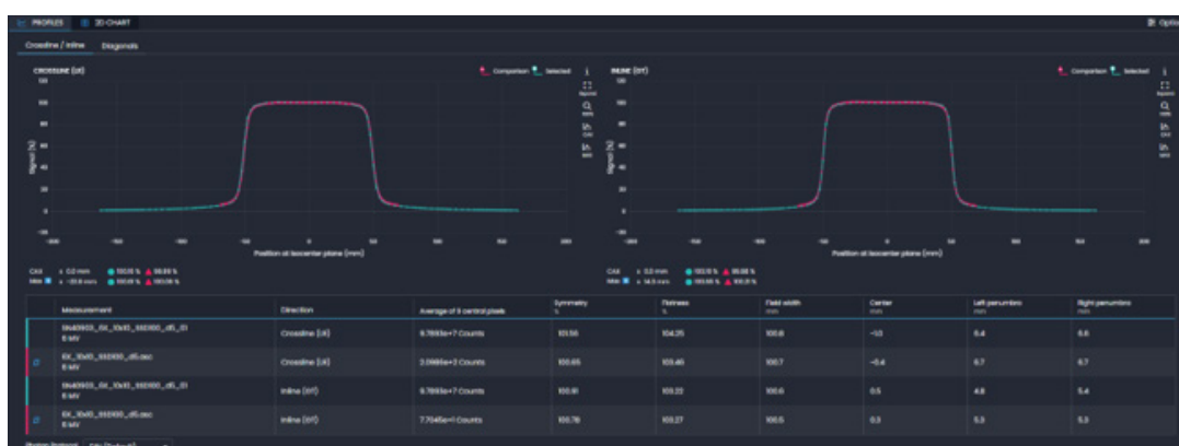
Figure 4. 6 MV 10 x 10 cm 2 at 5 cm water-equivalent depth, SDD = 100 cm, for water phantom (red) and myQA StarTrack3 (blue).
