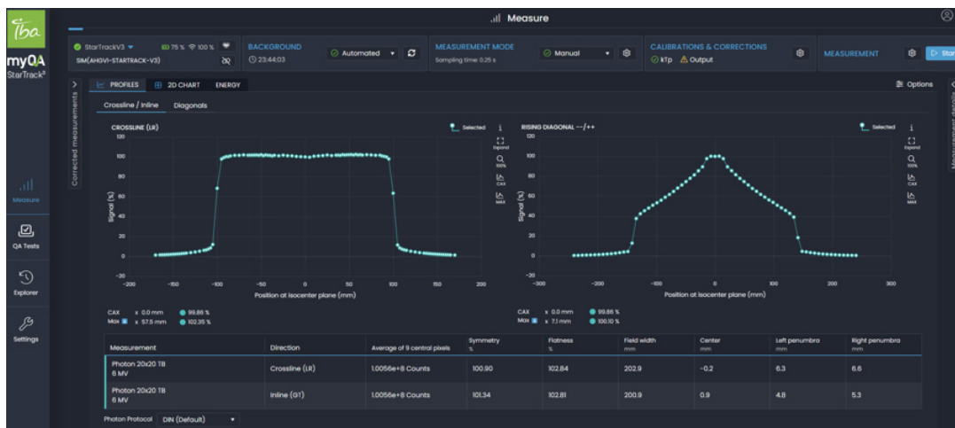
Figure 3. myQA StarTrack3 WebApp. A 6 MV 20 x 20 cm 2 field is irradiated through the photon energy verification plate. Profile features are assessed via DIN protocol (inline and crossline) while the diagonal wedge absorption is clearly visible.
